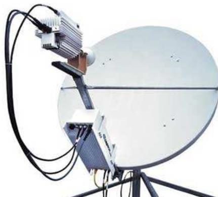
Antena Parabola VSAT
